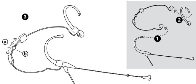
The donut-shaped moisture guard is provided to protect the element from sweat and moisture. Position the moisture guard as close to the element as possible to provide maximum protection. To remove the moisture guard, first remove the element cover and place it out of harm's way. Gently slide the moisture guard over the element. Replace the element cover.
