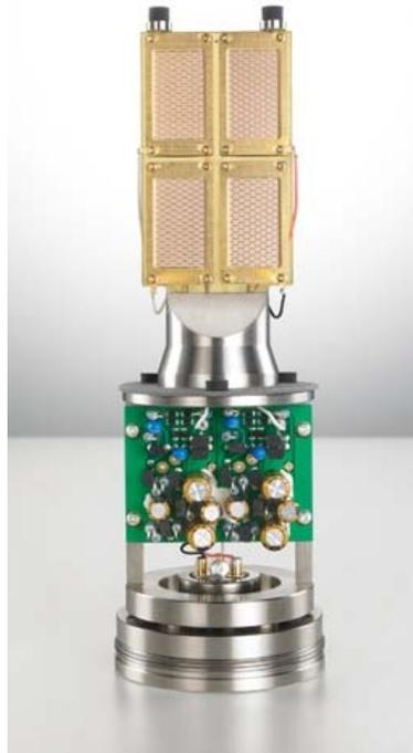
Since each part of the microphone body is rigidly connected and unified, we were able to eliminate the need for any components related to RFI countermeasures.
